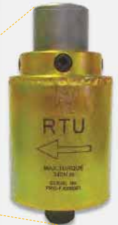
Modification of RTU for Track Bolt Tightening
